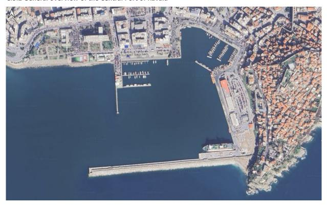
Currently, visiting cruise vessels berth at the south of the port basin, where two berths are available for cruise vessels: one large berth with a length of 470 m and a smaller berth with a length of 160 m (refer to image below). The latter is currently also used for ferry operations. The maximum available depth at the berths is  $\sim$ 8.8 m.
